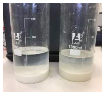
Lithium brines processed with aMES TM technology, as a pretreatment.
