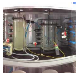
KLPP - potash brine preparation brine extraction for aMES™ processing)
