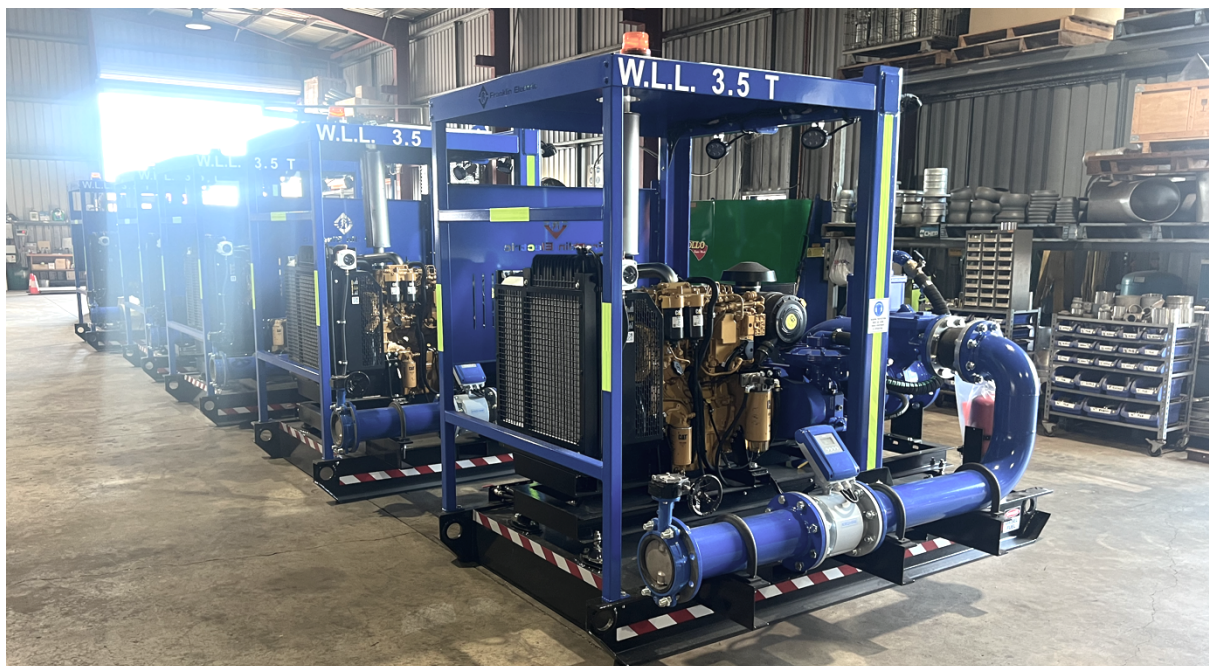
Figure 2: Industrial Diesel Pump Sets Supplied by PPS Undergoing Upgrades & Testing at PPS-Darwin
