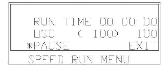
**Note:** All run menus will have two speeds listed. The leftmost speed will be displayed inside parenthesis. This is the target speed controlled by the user. The shaker will attempt to match this speed and should do so within ten seconds after making an adjustment. The rightmost speed is the tachometer reading, which shows the user what the shaker is actually running at. The tachometer is accurate within +/- 1% of actual speed.
