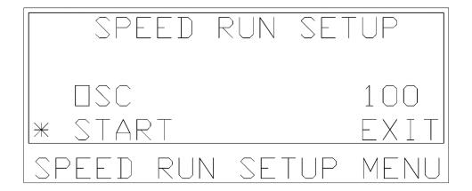
The user will now be taken to the speed run menu. The shaker will begin at the speed selected in the setup menu. The speed run menu behaves in the same way as the run menu with one exception. Pressing EXIT will not take the user back to the main menu instead pressing EXIT will take the user back to the speed run setup menu.
