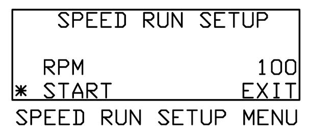
The user will now be taken to the speed run menu. The shaker will begin at the speed selected in the setup menu. The speed run menu behaves in the same way as the run menu with one exception. Pressing EXIT will not take the user back to the main menu instead pressing EXIT will take the user back to the speed run setup menu.
