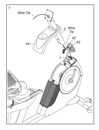
8. **Tip: Avoid pinching the wires.** Slide the Upright (2) onto the Frame (1).
