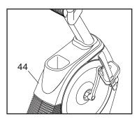
Next, using an adjustable wrench, turn the right pedal counterclockwise and remove it. Then, remove the screws from the right and left shields, and gently remove the right shield.
