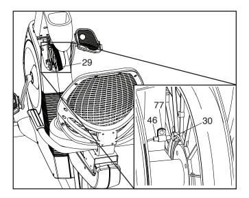
Then, retighten the M4 x 16mm Screw (77). Plug in the power adapter and turn the Pulley (29) for a moment. Repeat these actions until the console displays correct feedback.
