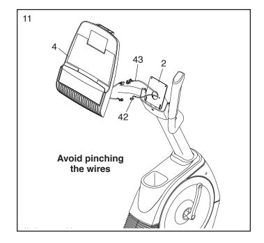
12. **Tip: Avoid pinching the wires.** Locate the two console screws in the back of the Console (4). Slide the console screws upward into the indicated slots in the Upright (2).
