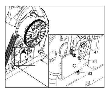
When the Drive Belt (47) is correctly adjusted, reattach the right shield, the right pedal, and the top shield and then plug in the power adapter.
