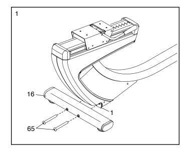
Set a sturdy piece of packing material under the front of the Frame (1). Have a second person hold the Frame to prevent it from tipping while you complete this step.
