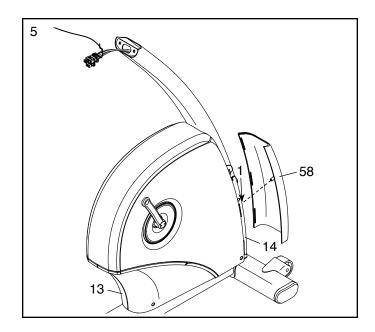
6. Orient the Upright Cover (57) as shown. Hold the Upright Cover near the Upright (2), and insert the wires upward through the Upright Cover.
