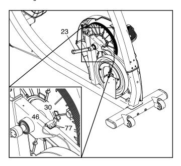
Plug in the power adapter, and turn the Right Crank Arm (23) for a moment. Repeat these actions until the console displays correct feedback.
