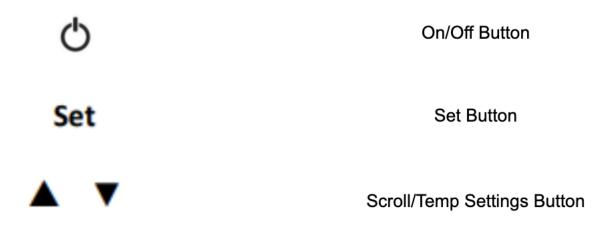
Switch the on/off button to turn the ice bath on. Press set to check/designate a temperature. Increase or decrease the temperature using the scroll/temp settings button, then select set again to lock in your new temperature. Switch off via the on/off button.
