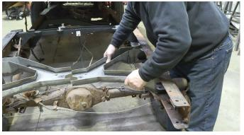
Install the support plate into the center, bridging the crossmember gap. The inner 4 holes will use the M8 hardware, and the outer 4 will take the M10x20mm
