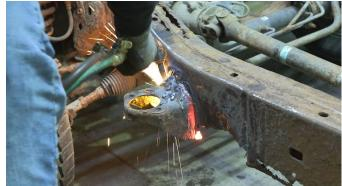
Clean and grind the rail free of rust and debris, revealing bare metal. Then spray the work area with a weldable primer to help prevent further rust development.
