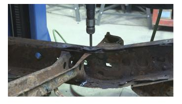
The top of the frame rail has a small lip. This will need to be slightly trimmed off in order to get the part into the channel.
