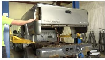
Remove your gas tank and EVAP system. If you wish to retain your factory gas tank strap, remove it at this time with a 12mm socket.
