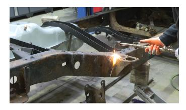
Grind away any remaining rust and debris revealing bare metal. Coat the part and work area with a weld-through primer to help prevent against further rust development.
