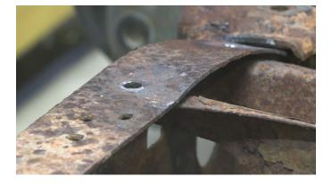
Grind away any remaining rust and debris revealing bare metal. Coat the part and work area with a weldthrough primer to help prevent against further rust development. Followed by painting the part and work area with a weldable primer to help prevent against rust development.
