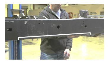
Grind the frame free of rust and debris, revealing bare metal.
