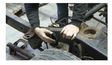
Tack weld the crossmember and shock mounts together. Then, following proper welding procedures, begin welding the part. 100% weld around all edges.
