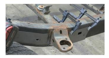
Remove any remaining potential fire hazards on both the vehicle and surrounding area. Following proper welding procedures tack weld the part onto the frame before welding the part on fully. 100% weld around all edges.
