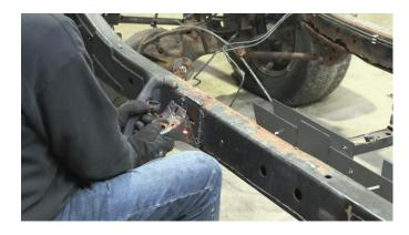
Hold the part up to the frame and mark off its coverage. Determine how much material you want to remove from the bottom, while leaving enough to weld back on to, and begin cutting.
