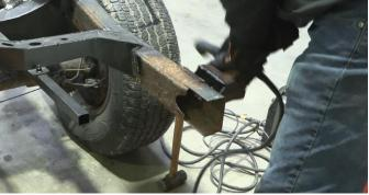
Hold the part up to the frame and mark off its coverage. Determine how much material you want to remove from the bottom, while leaving enough to weld back on to, and begin cutting.
