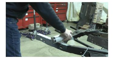
Push the part onto the frame while using the frame holes to help with alignment. C-clamp it into place.
