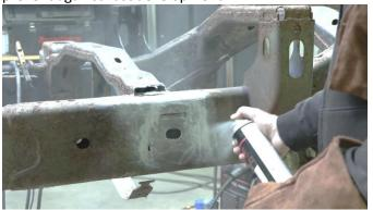
Using the silhouette where the factory cab mount was originally located, hold the part up to the frame and mark off its coverage using a paint marker.
