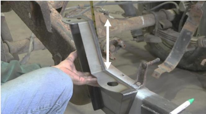
Use your measurements to align your body mount up with the opposite side. Once aligned, mark off its coverage using a paint marker.
