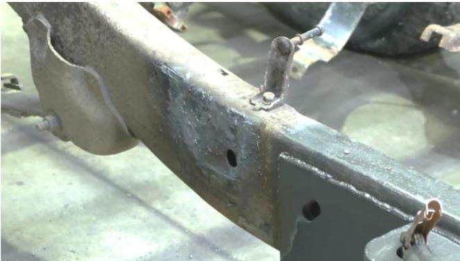
Grind the frame free of rust and debris.
