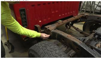
On the outside of the frame where the crossmember sits, there is a .5 inch hole that the factory uses as an alignment feature. Since we are removing this piece, we recommend drilling or marking this location so the new crossmember can sit in the factory location.
