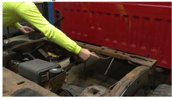
Mark off your cut lines and ensure you include the frame brackets.
