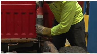
Remember to fully remove the brackets from the rails so that they're completely flush.
