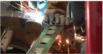
Finally, weld the included gas tank strap bracket to the frame rail.
