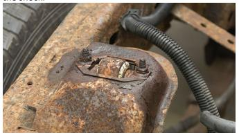
With a 21mm wrench and socket, remove the bottom bolt of the shock, and remove the shock.
