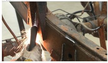
If you are not replacing your bed and body mounts, you will need to carefully remove them and reinstall later.
