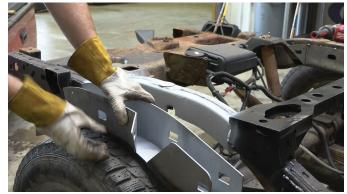
Push the part into place and C-clamp to the frame.
