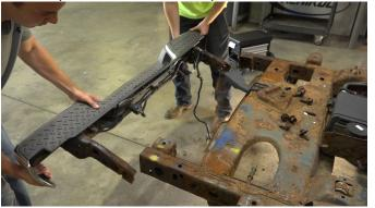
Slightly lift your vehicle to release some tension off of the leaf spring hanger bolt. With a 19mm and 21mm socket remove the bolt.
