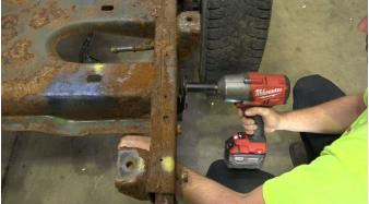
With a 21mm socket and wrench. Remove the rear shock bolt, and lift the vehicle to separate it the spring from the frame.
