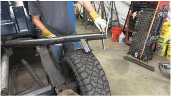
Put the remaining sheets on outside of the rails on each side of the vehicle, and C-Clamp them into place.
