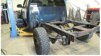
Unbolt the shock with a 21mm socket.
