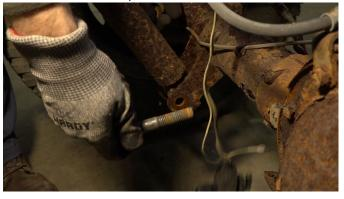
Begin punching out the rivets retaining the rear spring hanger. Support the vehicle and lower the axel. Remove the rear crossmember bolt from the bottom of the rail.
