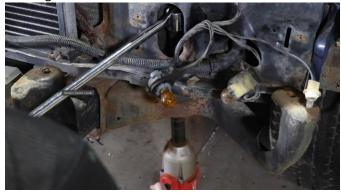
With an 18mm socket, remove the 5 bolts from inside the supports, and remove the bumper brackets.
