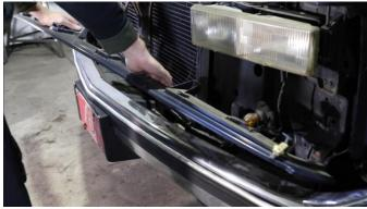
With an 18mm socket, remove the 8 bolts retaining the bumper, 4 on top and 4 on the bottom.
