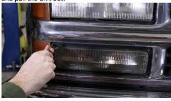
Remove the headlights and turn signal by pinch their plastic clips and rotating them out.
