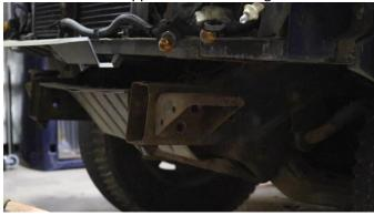
Begin cutting the mount from the frame. Clean the area of rust and debris, revealing bare metal.
