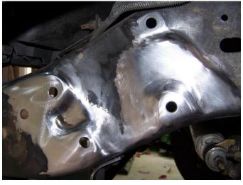
(OPTIONAL) Paint the part and work area with a weldable primer to help prevent against rust.
