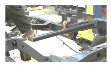
Then, slide the two remaining plates onto the outer side of your frame rail.
