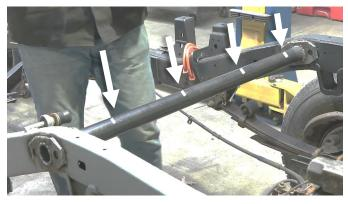
Once you have made your markings, hold your gas tank mount up to the crossmember and line it up with the two markings closest to the passenger's side. Make sure your mount is facing vertically. Tac weld it into place before welding it on fully.
