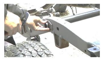
Following proper welding procedures, tac weld the inner and outer reinforcement plates into place, followed by welding them on fully.
