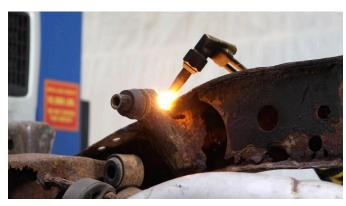
Begin cleaning the frame of any rust and debris, revealing bare metal.
