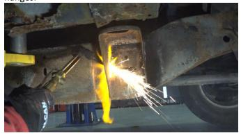
Clean the frame free of rust and debris, revealing bare metal, while leaving enough material to weld back onto.
