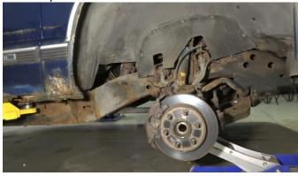
Remove any factory or aftermarket parts, linings, and/or coatings. Remove your leaf spring hanger bolt and bushing.
