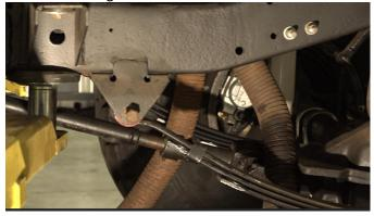
Remove your upper shock bolt, and detach the shock.
