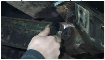
Cut as close as possible to the rear cross member and remove the remaining shackle mount material inside it.
