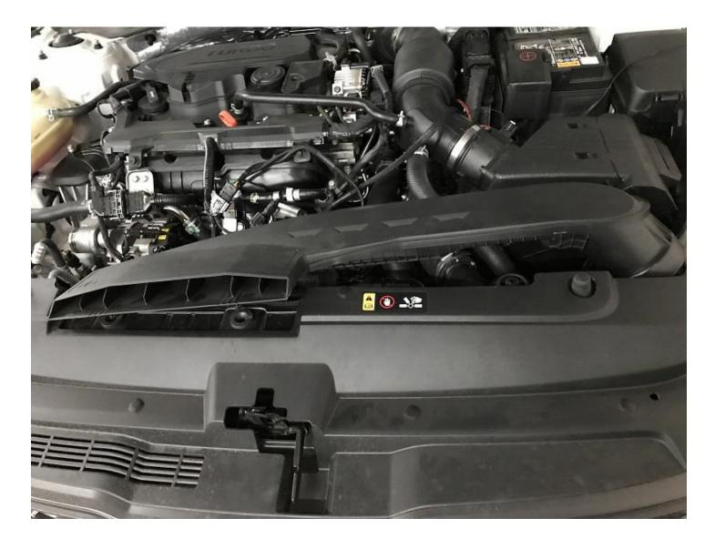
Pull down the squeeze clamps on the intake hose to diverter valve using pliers. Remove the hose and clamps going to the diverter valve. Store these away for when you want to put the car back to stock.
