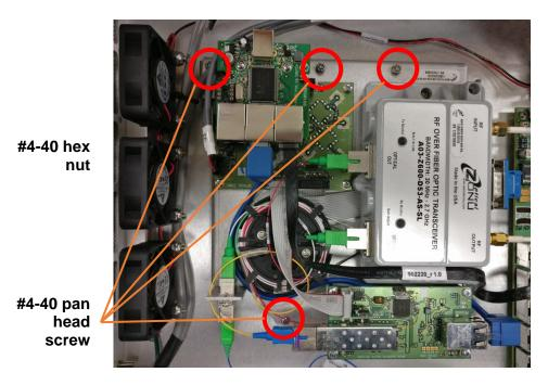
7. Reconnect the Ethernet cable, two (2) RF coaxial cables, fiber optic cable, and power cable to the Fiber Optic Unit.
