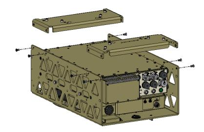
2. Remove twenty-eight (28) #6-32 truss head screws using a #2 Phillips Screw driver to remove the Lid.
