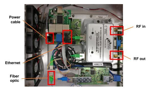
4. Remove three (3) #4-40 hex nut and one (1) #4-40 pan head screw using a 3/16" wrench and a #1 Phillips Screw Driver.
