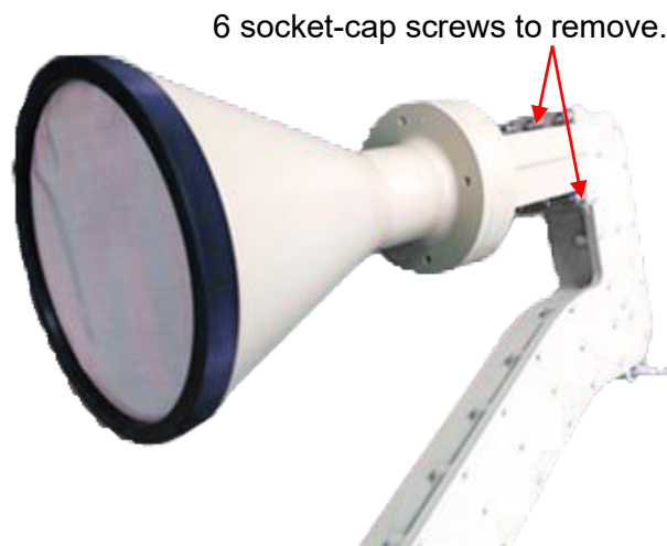
Figure 26: Location of the 6 socket-cap screws to remove.
