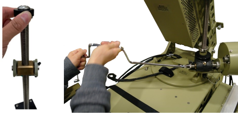
Figure 31: Adjust the Elevation Manually
