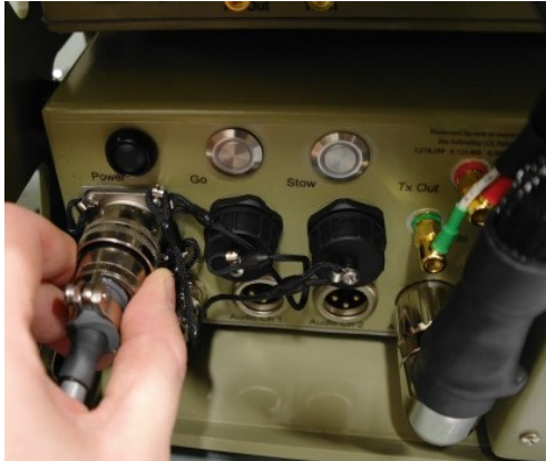
Figure 19: Connect LCD Touchscreen to Baseband
