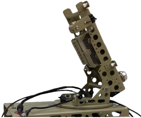
Figure 8: Install the Backplate onto the Baseband
