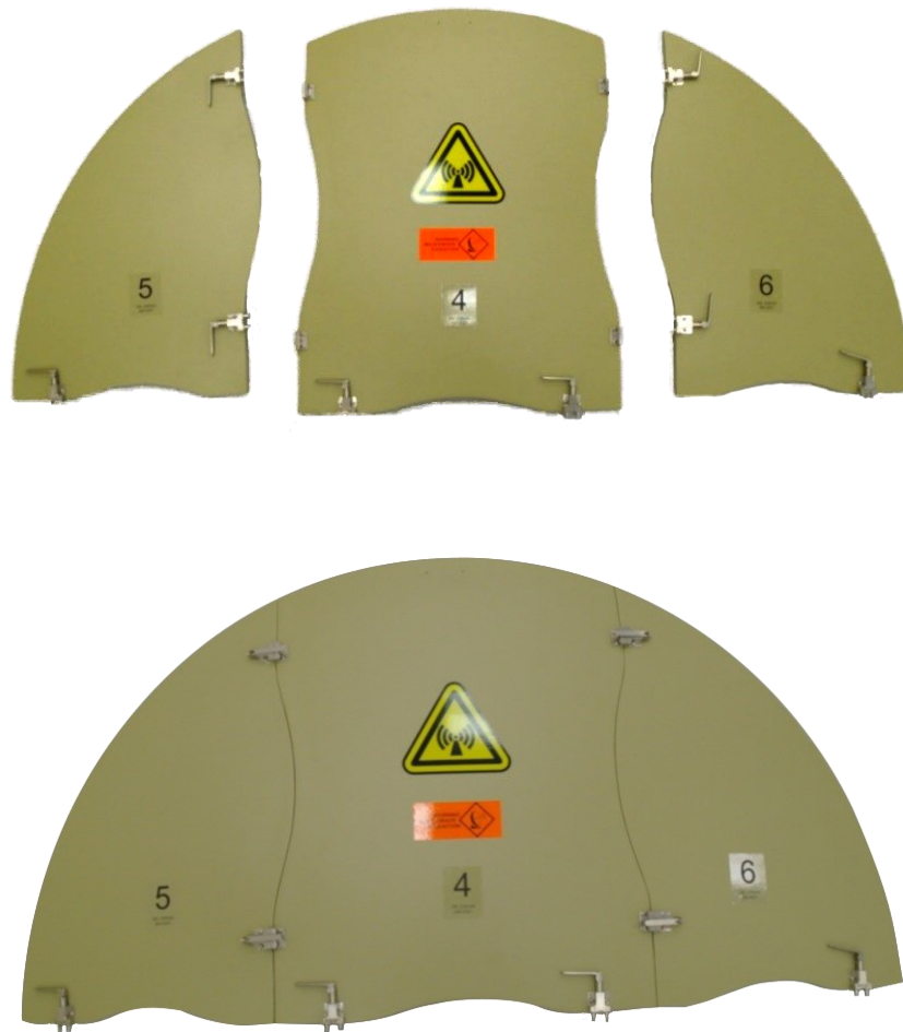
Figure 15: Assemble Segment 4,5, and 6 Reflector Petals together
