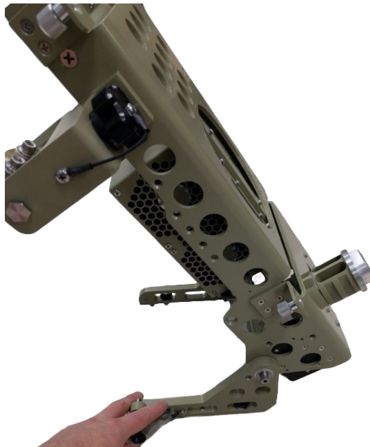
Figure 7: Fold the Supporting Arms of the RF Backplate
