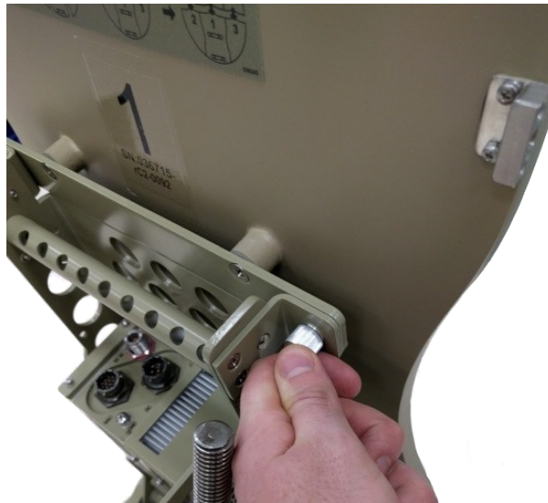
Figure 12: Secure Segment 1 Reflector Petal Using the Thumbscrews
