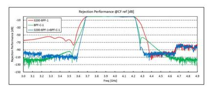
3200-BPF-1 LNB (LNB with integrated 5G filter), the BPF-C-1 (5G waveguide BPF) and the combination of the BPF and the LNB with integrated filter. In all cases the passband is 3.7-4.2 GHz.
