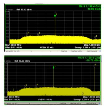
interference which will cause intermodulation products in the RF and mixer stages of the LNB. The 3200-BPF includes filtering at RF to mitigate this.
