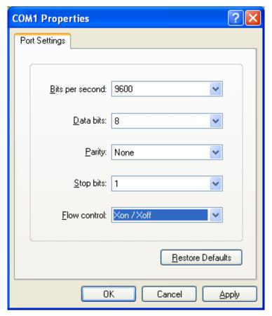
Figure 2-11: Setup Serial Port
