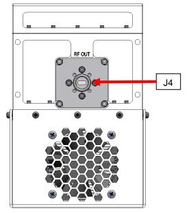
Figure 2-7 Standard Waveguide Output for ATOM Ka 50W units
