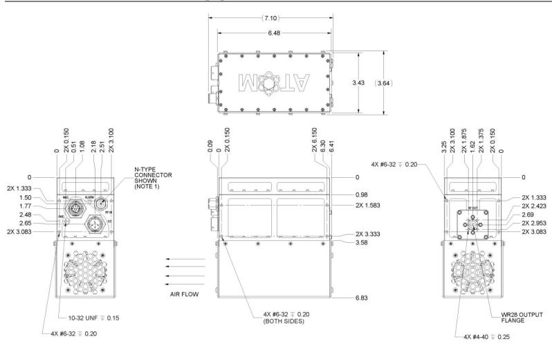
Figure A-3-1: 25W Ka BUC/SSPA, Fan Cooled
