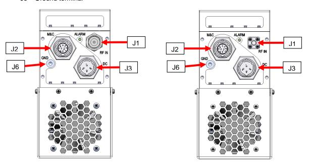
Figure 2-2 Input Connections for ATOM Ka 25W BUC Unit (N-Type Jack Shown)
