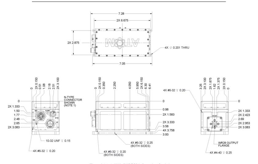
Figure A-3-2: 25W Ka BUC/SSPA, Baseplate Cooled
