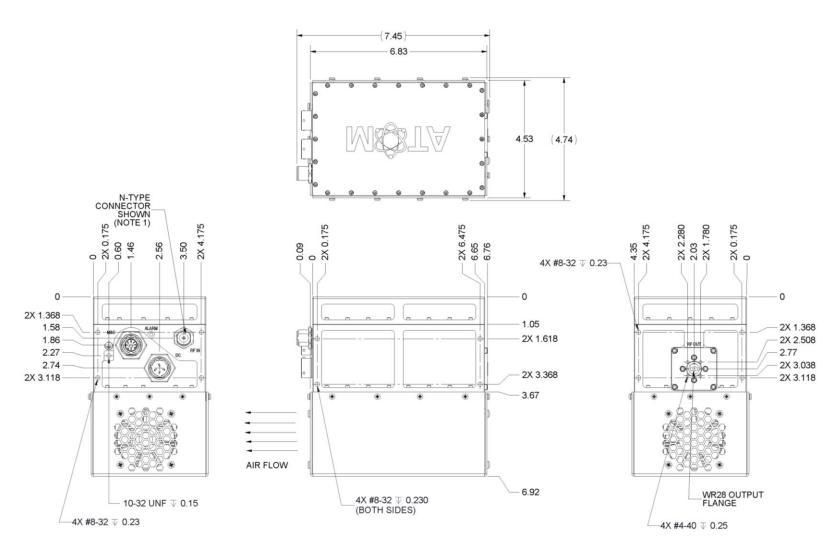
Figure A-3-3: 50W Ka BUC/SSPA, Fan Cooled
