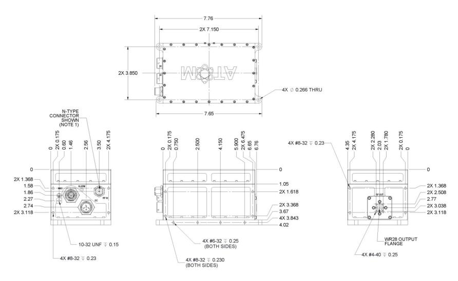
Figure A-3-4: 50W Ka BUC/SSPA, Baseplate Cooled
