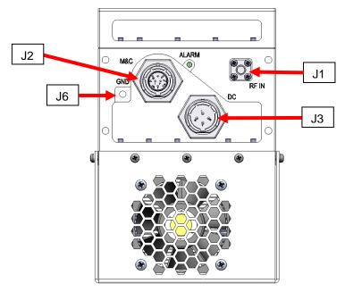
Figure 2-4 Input Connections for ATOM Ka 50W SSPA Unit
