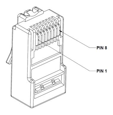
Figure 2-10: RJ-45 Plug Pinout
