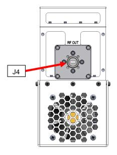
Figure 2-5 Standard Waveguide Output for ATOM Ka 25W units
