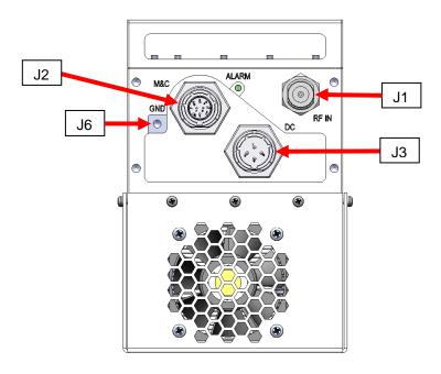
Figure 2-3 Input Connections for ATOM Ka 50W BUC Unit (N-Type Jack Shown)
