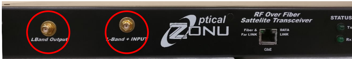
Figure 21: Tx and Rx Port on the External Modem
