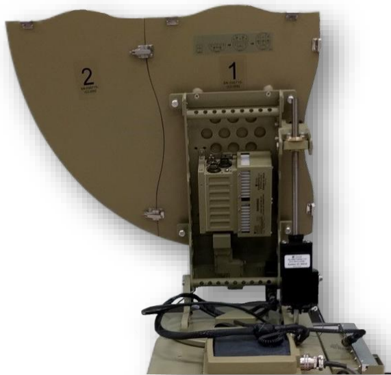
Figure 13: Install Segment 2 Reflector Petal
