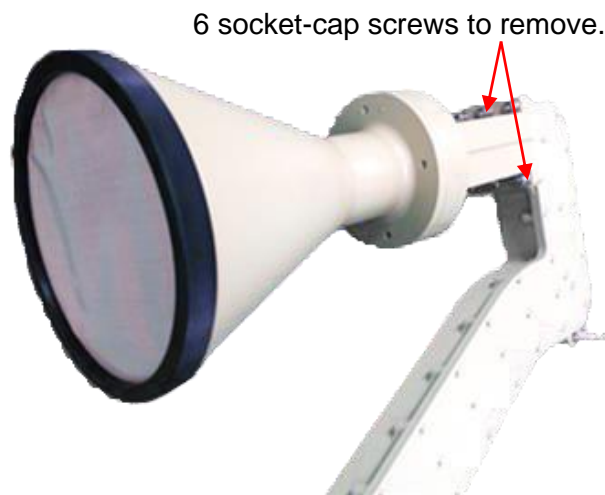
Figure 26: Location of the 6 socket-cap screws to remove.
