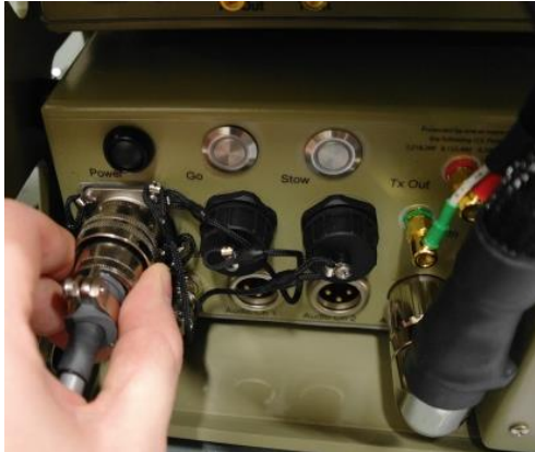
Figure 19: Connect LCD Touchscreen to Baseband
