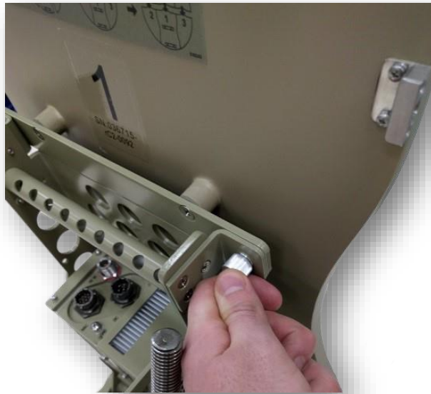
Figure 12: Secure Segment 1 Reflector Petal Using the Thumbscrews
