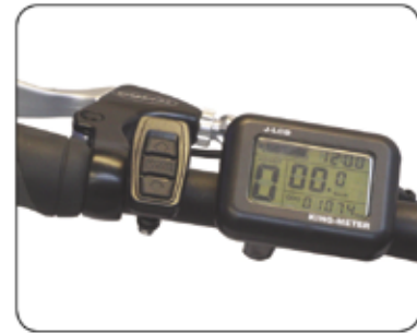
Fig. 9.3 King Meter® Display, Set "ASSIST" to "0" While Programming
