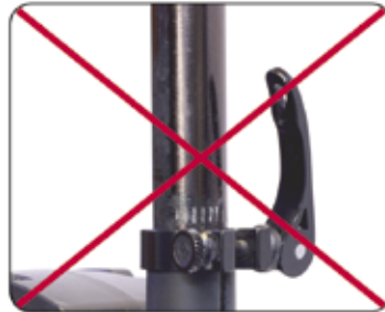
Fig. 4.2 Incorrectly Installed Seat Post
