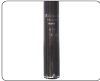
Fig. 4.1. Seat Post, "Minimum Insert Line"
