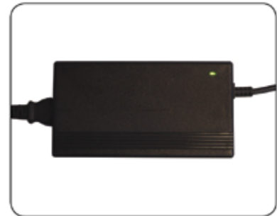
Fig. 7.4 Battery Charged - Green LED
