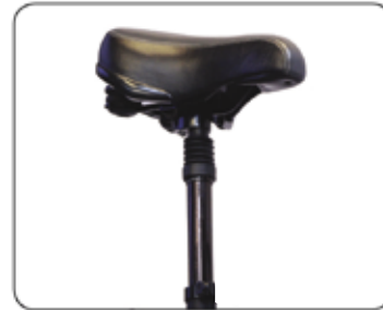
Fig. 4.3 Seat Post Inserted Correctly, Past "Minimum Insert Line"
