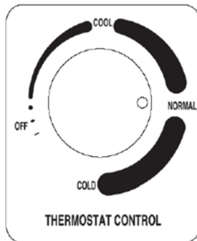
4. The thermostat controls compressor's "ON/OFF" by sensing inside temperatures of cabinet.
