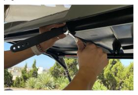
**STEP 6.** For upper roll bar installations use Step 5 with Metal Brackets (5). Install Particle Separator (1) onto the Metal Brackets (5) on the left and right-side using Bolt (6) and Washer (4) and a 3/16" standard wrench to tighten. Washer **MUST** be between the Metal Bracket (5) and Particle Separator (1). If the washer is placed under the head of the Bolt (6) the Particle Separator will rotate freely and may cause damage.
