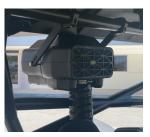
**STEP 7.** Measure the flex hose ducting (8) to the Particle Separator (1), *if necessary*, cut excess off the Flexible Hose Duct (8) with wire cutters or scissors. NOTE: pull 1" of the internal wire from the top of the hose for a secure fit to the Particle Separator (1). Insert the Hose Clamp (2) over the end of the Flexible Hose Duct (8) that is sticking out of the Air Intake cover. Place the Flexible Hose Duct (9) over the Particle Separator (1) intake and tighten with a Philips screwdriver.
