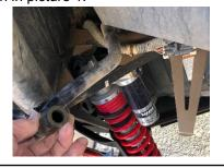
**STEP 3.** Insert duct coupler (8) into the flex hose (9). Add two hose clamps (2) over the flexible hose (8) and the duct coupler (8). Insert duct coupler (8) and flexible hose (9) into the intake airbox. Tighten one hose clamp (2) over the duct coupler and one hose clamp (2) over the flex hose (9).
