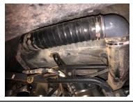
**STEP 4.** You will now cut a 4" hole behind the driver seal on the sidewall corner of the bed (see photo 1), using a 4" diameter hole saw or trim using a dremel. Install included rubber stripping around the hole in the air plastic panel. Insert the flexible hose (9) through the hole and attach to the stock tube that was revealed when taking out the plastic box.
