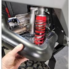
**STEP 5.** Insert the KWT Flexible Hose Duct (8) onto the stock RZR Filter Air Box intake and tighten the Hose Clamp (2) as shown below.
