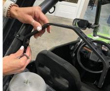
**STEP 3.** Install Particle Separator (1) onto the Hanger Bracket (5) on each side using Hex Head Screw (6) and Lock Washer (4). The lock washer **MUST** be between the Hanger Bracket (5) and Particle Separator Side Mount (3). If the washer is placed under the head of the Bolt (6) the Particle Separator will rotate freely and may cause damage.
