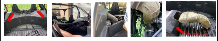
**STEP 3.** Remove push pins from the side intake and remove side intake.
