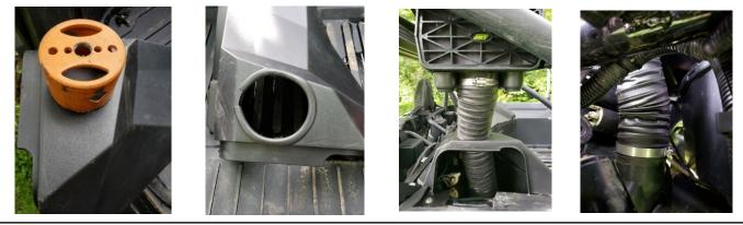
STEP 7. Re-check hose configuration for fit. Re-install Side Intake and install is complete.
