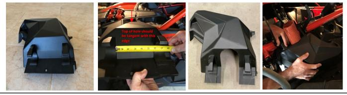
**STEP 5.** Install Particle Separator (1) onto the Metal Brackets (5) on the left and right-side using Bolt (6) and Washer (4) and a 3/16" Allan wrench to tighten per torque guide on page 1. Washer **MUST** be between the Metal Bracket (5) and Particle Separator (1). If the washer is placed under the head of the Bolt (6) the Particle Separator will rotate freely and may cause damage.
