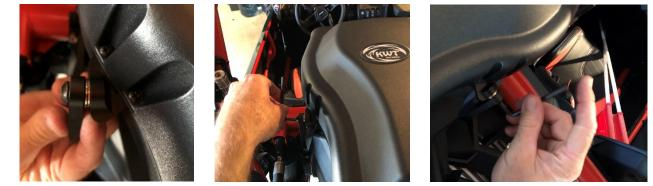
**STEP 6.** If necessary, cut excess off the Flexible Duct (9) with wire cutters and scissors for a better fit. NOTE: Pull 1" of internal wire out from the top of the hose to ensure a tight fit around the Particle Separator (1). Insert the Hose Clamp (2) over the end of the Flexible Duct (9) that is sticking out of the Air Intake cover. Place the Flexible Duct (9) over the Particle Separator (1) intake and tighten with a Philips screwdriver.
