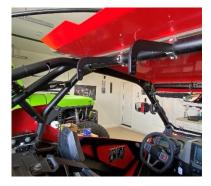
**STEP 3.** Install Particle Separator (1) onto the Metal Brackets (5) on the left and right-side using Bolt (6) and Washer (4) and a 3/16" allen wrench to tighten. The washer **MUST** be between the Metal Bracket (5) and Particle Separator (1). If the washer is placed under the head of the Bolt (6) the Particle Separator will rotate freely and may cause damage.
