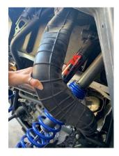
**STEP 5.** Insert the Flexible Hose Duct (8) onto the stock RZR Filter Air Box intake side and tighten the Hose Clamp (2) as shown below.
