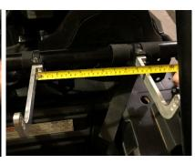
**STEP 3.** Take the stock Air Intake Cover and measure a hole that will align with the air intake. Cut a hole using a 3.75" diameter hole saw or trim using a dremel. Install included rubber stripping around the hole in the Air Intake Cover. Insert the Flexible Duct (8) through the Air Intake Cover and insert two Hose Clamps (2) over the end of the Flexible Hose Duct (9)
