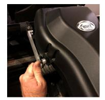
**STEP 7.** If necessary, cut excess off the Flexible Duct Hose (8) with wire cutters for better fit. Insert the Hose Clamp (2) over the end of the Flexible Duct Hose (8) that is sticking out of the Air Intake cover. Place the Flexible Duct Hose (8) over the Particle Separator (1) intake and tighten with a Philips screwdriver.
