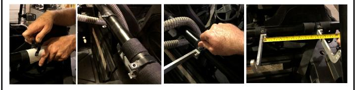
**STEP 3.** Take the stock Air Intake Cover and measure a hole that will align with the air intake. Cut a hole using a 3.75" diameter hole saw or trim using a dremel. Install included rubber stripping around the hole in the Air Intake Cover. Insert the Flexible Duct (8) through the Air Intake Cover and insert two Hose Clamps (2) over the end of the Flexible Hose Duct (9)
