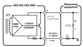
2-Wire Transmission method(Loop powered) using P/S(+ side) of Measuring equipment
