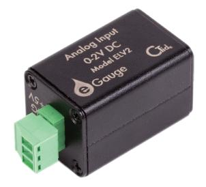
The eGauge 2V Analog Input Sensor allows EG4xxx meters to read 0 - 2V analog values or dry contact states from standard 2-wire dry contacts such as relays. The Analog Sensor requires the eGauge Sensor Hub (ESH044). Wiring diagrams for the Sensor Hub and compatible sensors can be found on the following page.
